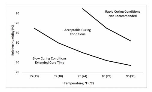
Aeroglaze Z306 coating cures to a tack-free surface in 2-3 hours at 25°C (77°F) and 50% relative humidity. Room temperature cure times of 12 hours permit handling.
