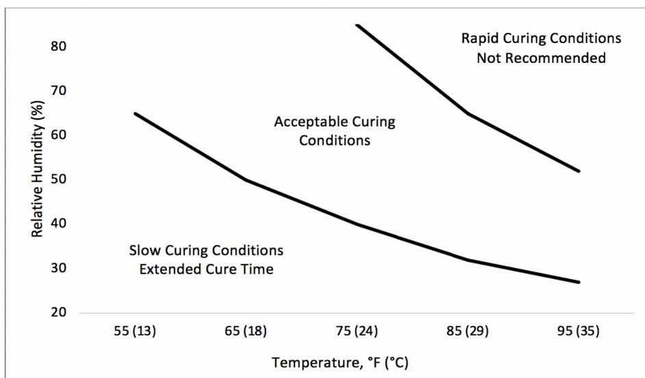
Chemglaze V022 cures to a tack-free surface in 2-18 hours at room temperature depending on the application thickness, catalyst, and relative humidity. Faster handling times can be achieved by using one of the following cure cycles:
