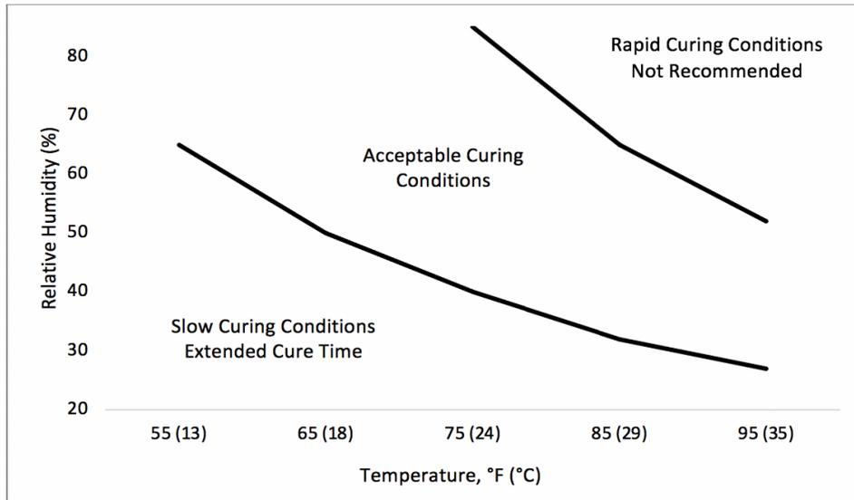
Chemglaze Z051 cures to a tack-free surface in 2-3 hours at 25°C (77°F) and 50% relative humidity. Room temperature cure times of 12 hours permit handling.
