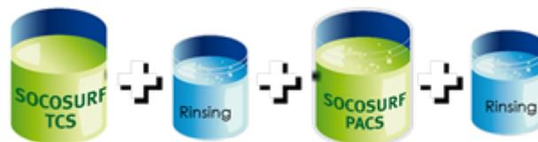
The **SOCOSURF TCS** is a trivalent chromium (Cr(III)) solution, and the Socosurf PACS is a post-treatment solution that reinforces the TCS coating.
